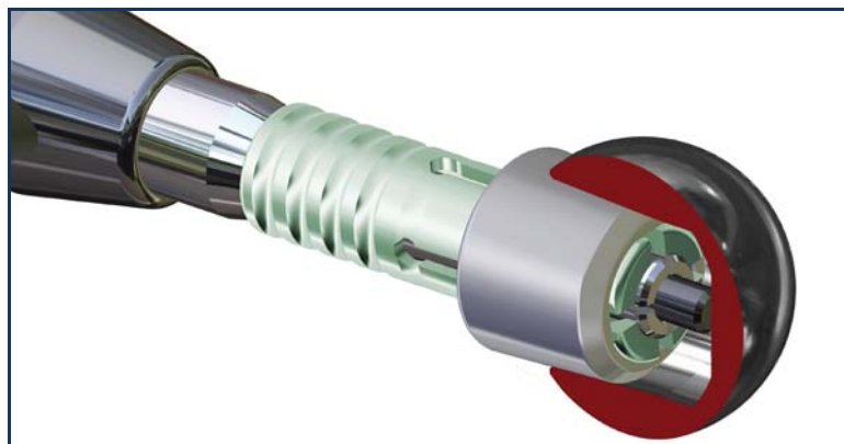
fig. 16: Use of the adapter extractor with extractor sleeve
